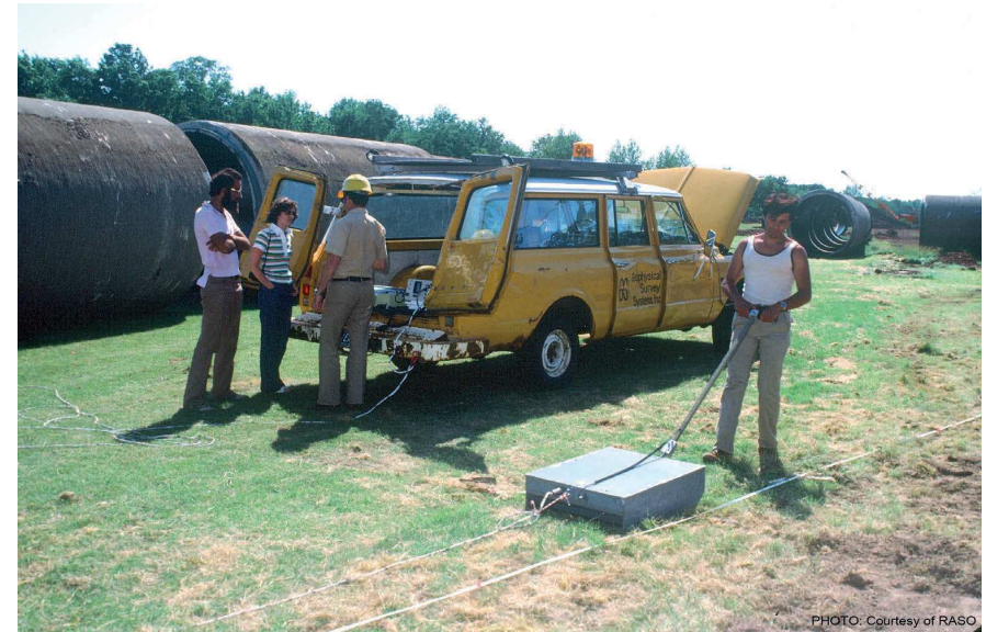
Plate 1. Geophysicists including Bruce Bevan of Geosight of New Jersey and from the firm of Geophysical Survey Systems of New Hampshire, pulling a prototype 300 MHz antenna capable of “seeing” through the cap of surface deposits and shale fill covering the buried settlement of Raritan Landing. The Ground Penetrating Radar equipment required a truck for transport in 1978; modern systems now fit into a backpack (Photo by Joel W. Grossman).
